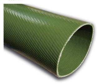
Oilvey 10 is one type of through-the -weave polyurethane (PU) covered hoses. Oilvey 10 hoses shall be made from 100% high tenacity synthetic yarn circular woven and completely, totally embedded in the PU compound, excellent protected against mechanical damage, forming a single homogenous construction without the use of any glues or adhesives of any type. Incorporated copper wire is used to transfer static electricity.
