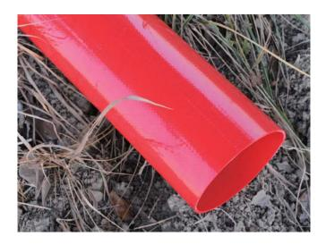
Manureflow is one type of through-the -weave polyurethane (PU) covered hoses. Manureflow hoses shall be made from 100% high tenacity synthetic yarn circular woven and completely, totally embedded in the PU compound, excellent protected against mechanical damage, forming a single homogenous construction without the use of any glues or adhesives of any type. Thick and smooth cover and super adhesion between layers ensure a long life span of drag hoses.
